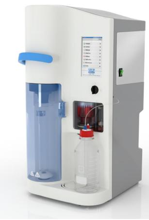
The UDK 159 Distillation & Titration System is designed to perform nitrogen and protein content according to the Kjeldahl Method (TKN) in the Food & Feed industries and several other applications in environmental control (phenols, nitrogen in water, sludge, soil and lubricant) and also in the chemical and pharmaceutical industries after having digested the sample accurately.
